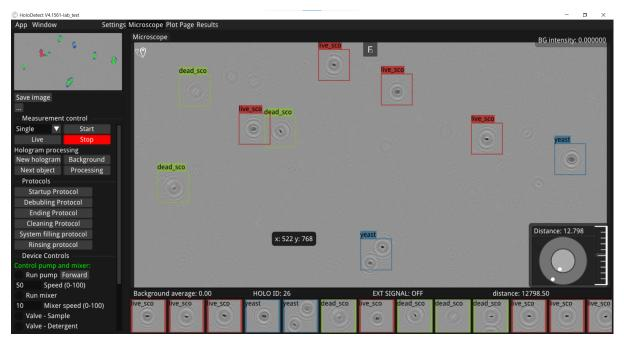
By clicking the central Fluor icon (capital F) the fluor display will also appear next to the hologram. The centers of the measured fluorescent and hologram objects should be aligned.
