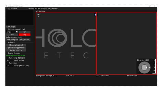
Double-click on the holographic image to display both the holographic and fluorescence images at full size.
